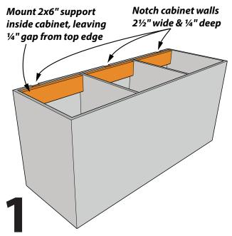
The cabinet must be reinforced with a 2x6". Space the brackets 18-24" apart, starting 3-6" from the outer edges. Ensure brackets sit flush with cabinet.
