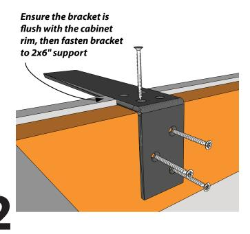
Determine if included screws are appropriate for your project. Fasten brackets to support using 4 screws per bracket.
