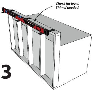
Check that the brackets are level and glue shims onto the brackets as necessary
