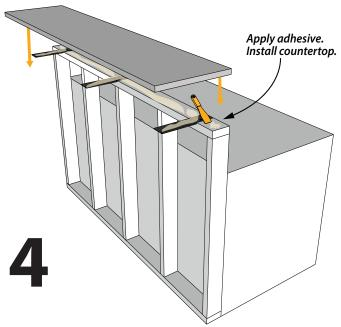
Use an appropriate epoxy or construction adhesive to mount the countertop.
