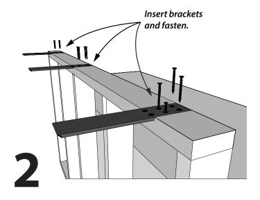
Determine if included screws are appropriate for your project. Fasten brackets to support using 4 screws per bracket.
