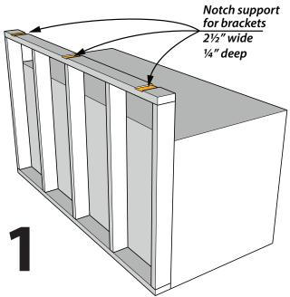
Space the brackets 18-24" apart, starting 3-6" from the outer edges. Ensure brackets sit flush with support.
